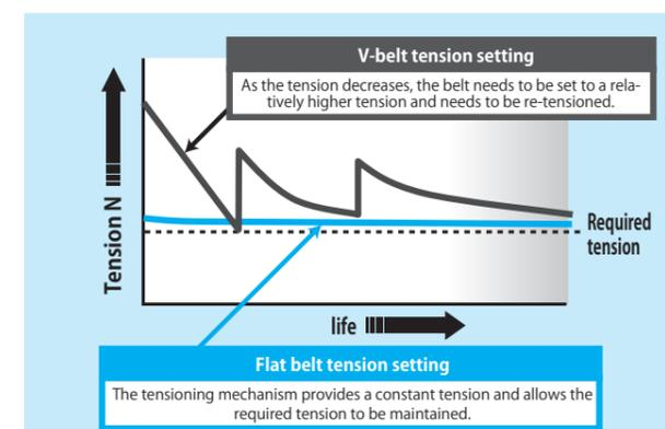
As the flat belt is thin, it is less affected by bending distortion when it is wrapped around a pulley. Therefore, even if it is affected by reverse bend, its service life is as long as approximately 2.5 times that of V-belts. The tensioning mechanism eliminates the reduction in tension that used to occur with V-belts and allows a tension close to the required tension to be maintained at all times; making the belt maintenance-free and achieving a longer service life.
